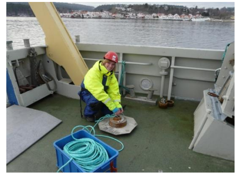
Figure 6: Securing the flux chambers with rope before placement on the sea bed
