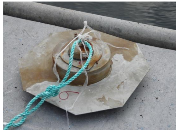
Figure 17: Flux chamber with POM attached, measuring free aqueous concentration, C_w
