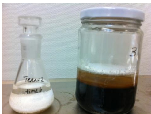
Figure 13: Tenax extraction (left) and tenax as an infinite sink (right).
