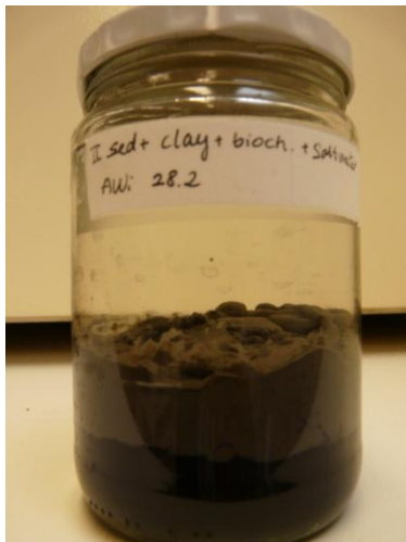
Figure 10: Too thick clay caused lumps and unevenness
