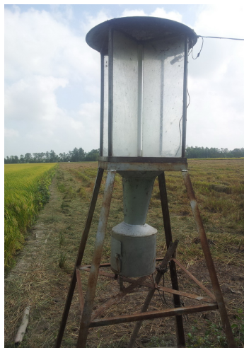
Figure 10: The insect monitoring light trap to predict damage of Nivaparvata lugens species for the Globalgap rice production
