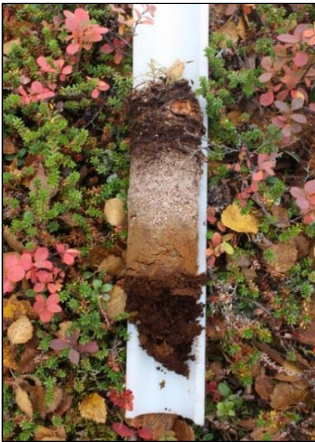
Figure 6. An example of a soil core sampled from the poorly podzolized soil (P1).
