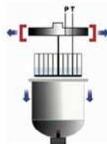
Clamp is released and sample rack automatically rises from chamber
