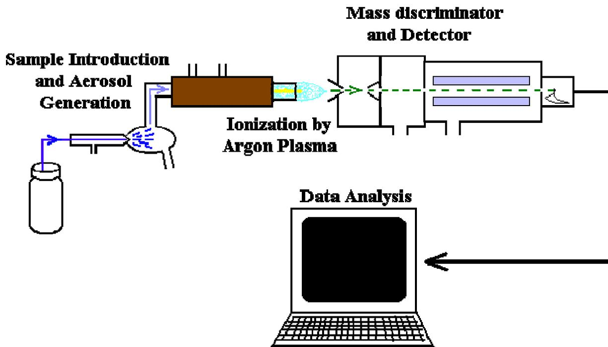
**Figure 6 : Schematic of ICP-MS main processes** (Steve Kvech, <http://www.cee.vt.edu/ewr/environmental>)
