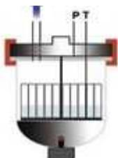
Fast cooling step due to water cooling of chamber. Chamber is vented and acid vapors extracted
