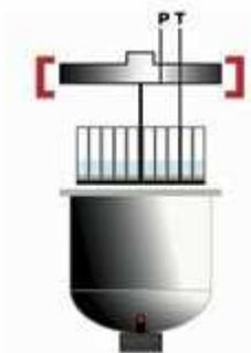
Sample rack is lowered automatically into microwave chamber
