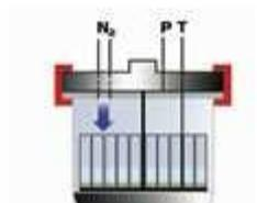
Chamber is pressurized with N<sub>2</sub> prior to start of run – prevents any boiling of samples – cross contamination is eliminated
