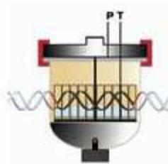
Microwave energy is applied. All samples under same temperature and pressure conditions
