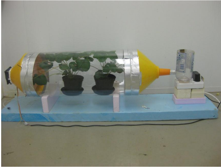
Figure 2. Tunnel with plants with N. floridana inoculated T. urticae and a spore trap.
