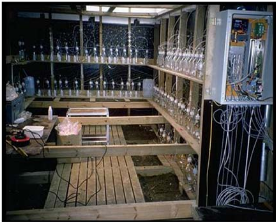
Figure 8: A) Picture inside the lysimeter trench (French 1999). B) Sketch showing the principle behind the suction cups extracting water at the lysimeter trench at Moreppen. Suction is created by the vacuum pump in the Prenart soil water sampler (location of the samples shown in figure 7 and water is extracted from the soil profile and collected in the Prenart collecting bottle.
