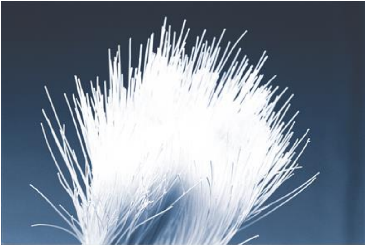
Figur 10 "Hollow fiber"-membraner (Hangzhou H-Filtration Membrane TEchnology & Engineering CO Ltd. 2013)
