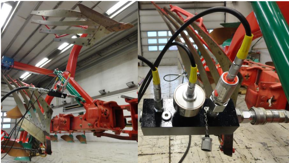
Figure 8.41 (left): The plough body fully released at the end of the first lift phase of the release sequence subject to this test
