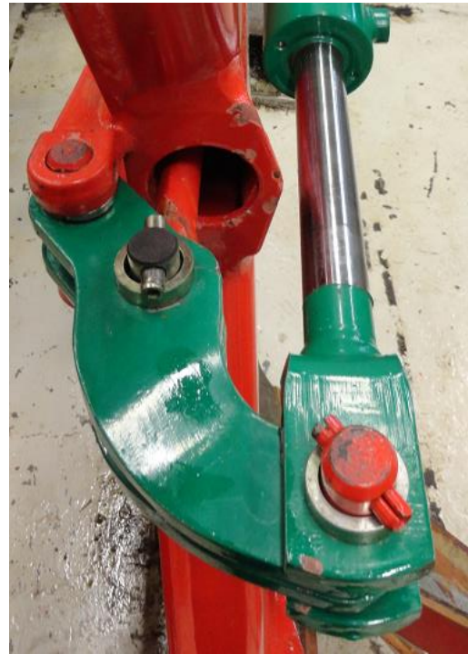
Figure 8.16 (left): This is how the mechanical system with tie plates and cylinder turned out on the plough beam.
