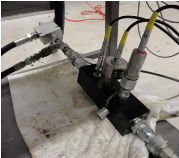
Figure 8.43: Relocation of pressure-, flow and oil temperature measurement to obtain conditions by pressure relief valve for the second part of the measurements regarding phase 1 (plough body lift) of the release sequence. Note that the accumulator is removed.
