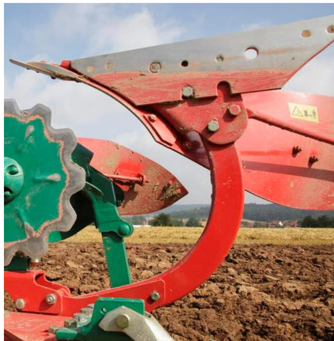
Figure 1.3 (left): Kverneland Auto Reset System with the leaf spring coloured green.
