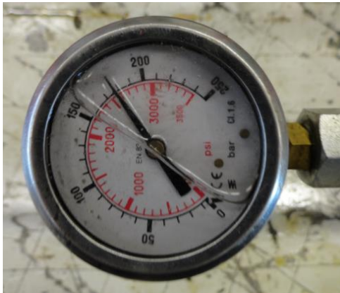
Figure 8.36 (left): Cylinder pressure during test was 180 bar, equivalent to 17 kN of force-on-point during the release sequence.
