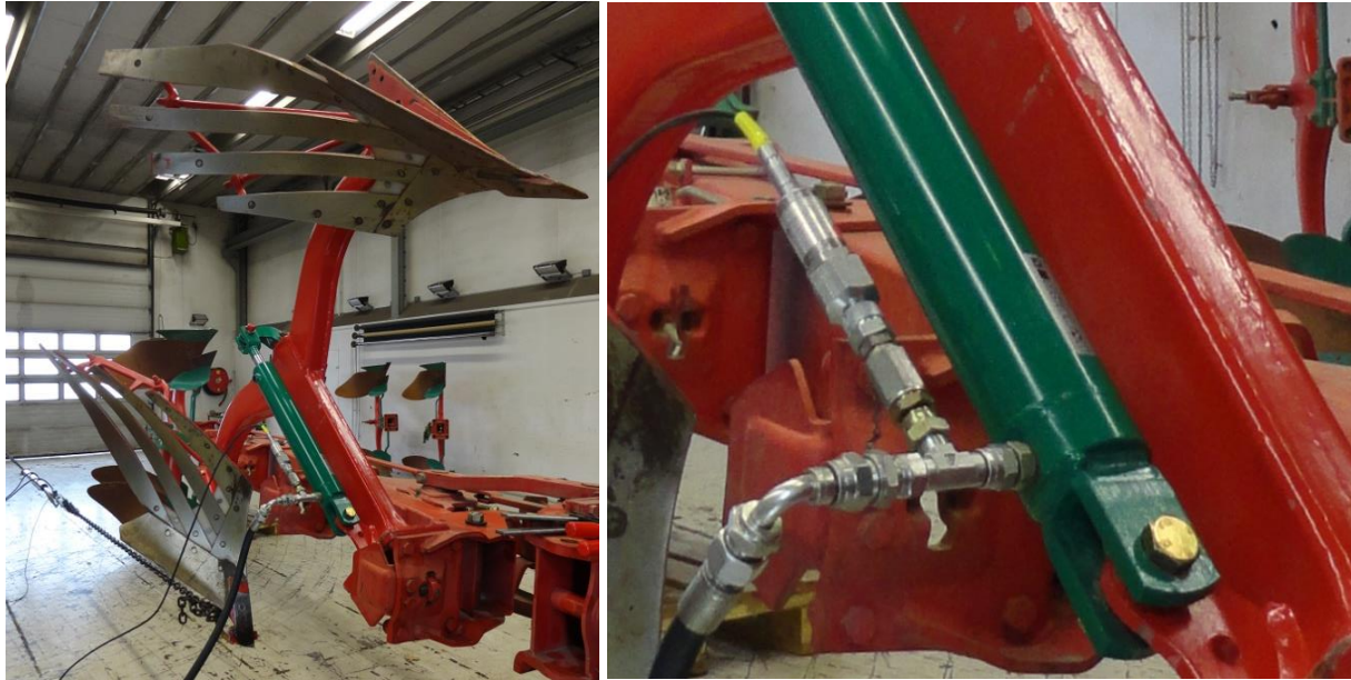
Figure 8.31 (left): The plough body fully released, during test of mechanical release characteristics.
