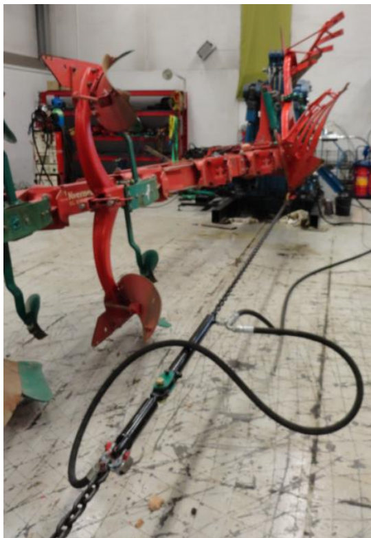
Figure 8.38 To pull the plough point, two hydraulic cylinders with dimensions D40-d20 was connected with chains to it. The cylinders were chosen with a cross-sectional area as small as possible in order to get as much velocity on the plough point as possible out of the oil delivery from tractor rig. In order to get sufficient stroke length two cylinders were connected in series with a total stroke length by 650 mm.
