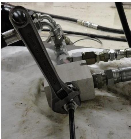
Figure 8.22: To avoid that the pressure relief valve burst and interfere on the pressure adjustment measurements, the mechanical spring is tensioned to maximum burst pressure, which is rated to 400 bar in product leaflet, according to (Comatrol-2 2010). Illustration by own photo.
