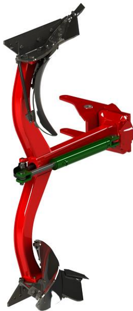
Figure 7.40 (left): Rendered image of the mechanical design of the system connected onto the plough beam.
