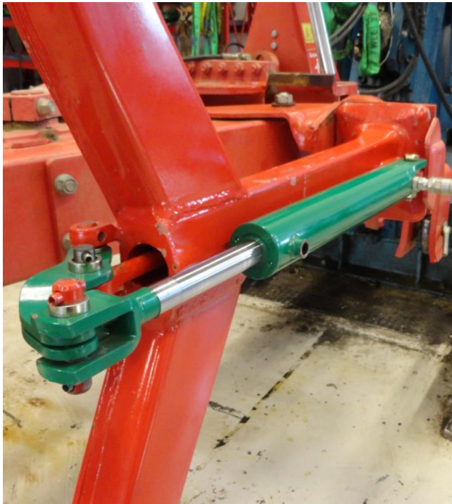
Figure 8.16 (left): This is how the mechanical system with tie plates and cylinder turned out on the plough beam.
