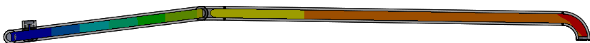
Figure 7.13: As seen from this illustration the results output indicates a pressure deviation or rather pressure loss through the pipeline of 8 bar. The (red) 168 bar pressure indication at 90° elbow at cylinder outlet, shows the pressure in the beginning of the pipeline, while the (blue) 160 bar pressure indication at valve connection shows the pressure at the end of the pipeline.
