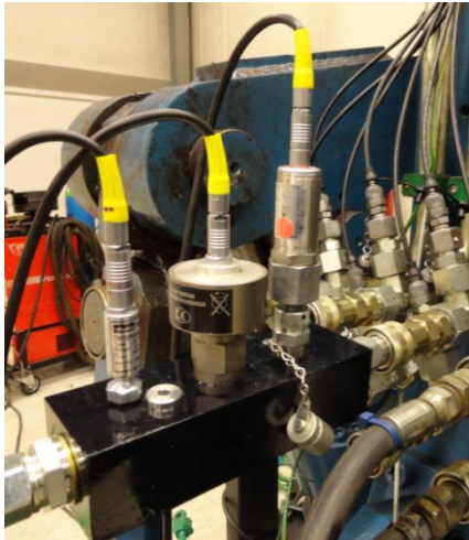
Figure 8.20: To keep track of the inlet flow into the directional valve, oil flow delivery from the tractor outlet was measured. Illustration by own photo.
