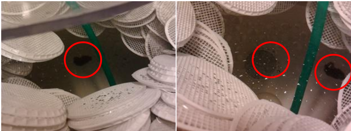
Figure 4.20: Undissolved starter fish feed at the bottom of individual setups B5 and B6, two day after addition on day 15 (Holdhus 2012).
