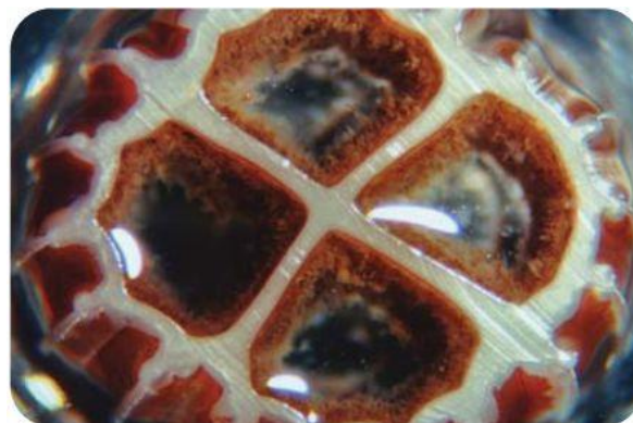
Figure 2.2: Close up photo of carrier type K1 with mature biofilm (Veolia 2011).
