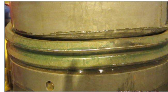
Figure 303: Original Split Lock Ring. [2]
