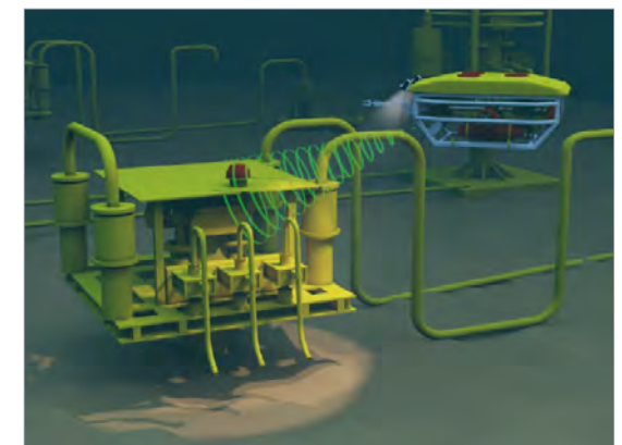
Figure 197: WFS's wireless communication system for subsea. [39]
