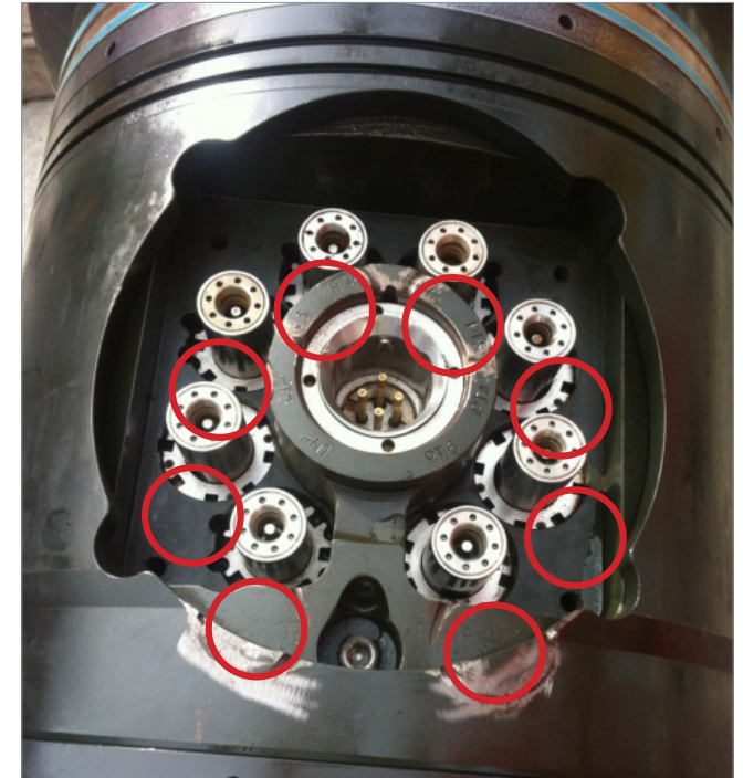
Figure 307: Red circles indicating where the Hybrid Penetrator got engaged into the TH. [2]
