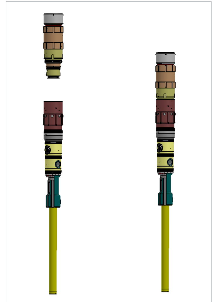
Figure 28: While the THRT is in Unlatch-Unlock position, the THRT is lowered down into the TH. Scale of figure is about 1:50. [6]
