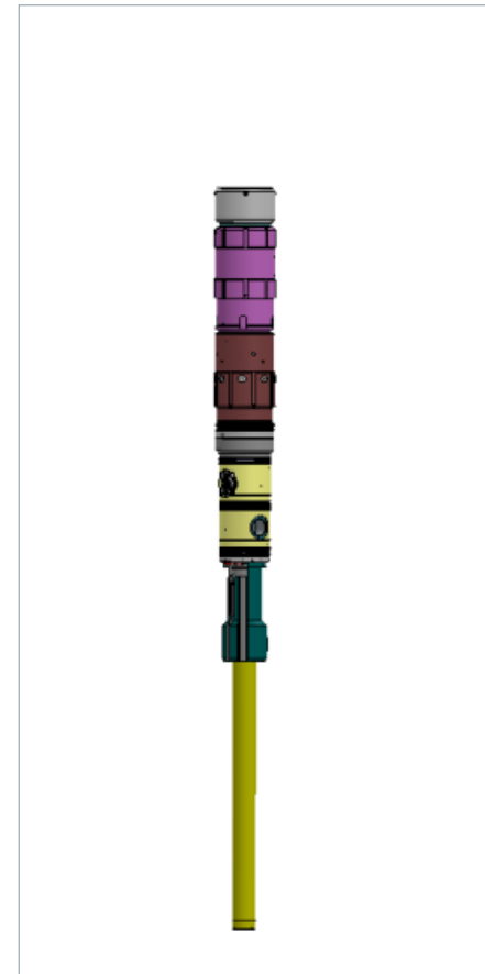
Figure 30: THRT is latched to TH. [6]
