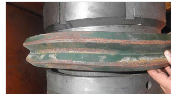
Figure 304: Deformed Split Lock Ring. [2]
