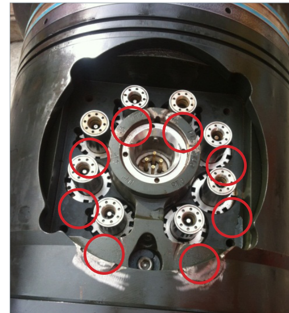
Figure 141: Red circles indicating where Hybrid Penetrator got engaged into TH. [2]
