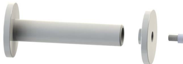
Fig 3.32 The final solution. A pin with a circular bracket and a socket head cap bolt.
