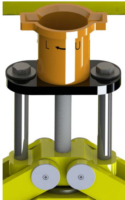
Fig 3.43 Support bracket for the ROV bucket. Mechanism in closed position.
