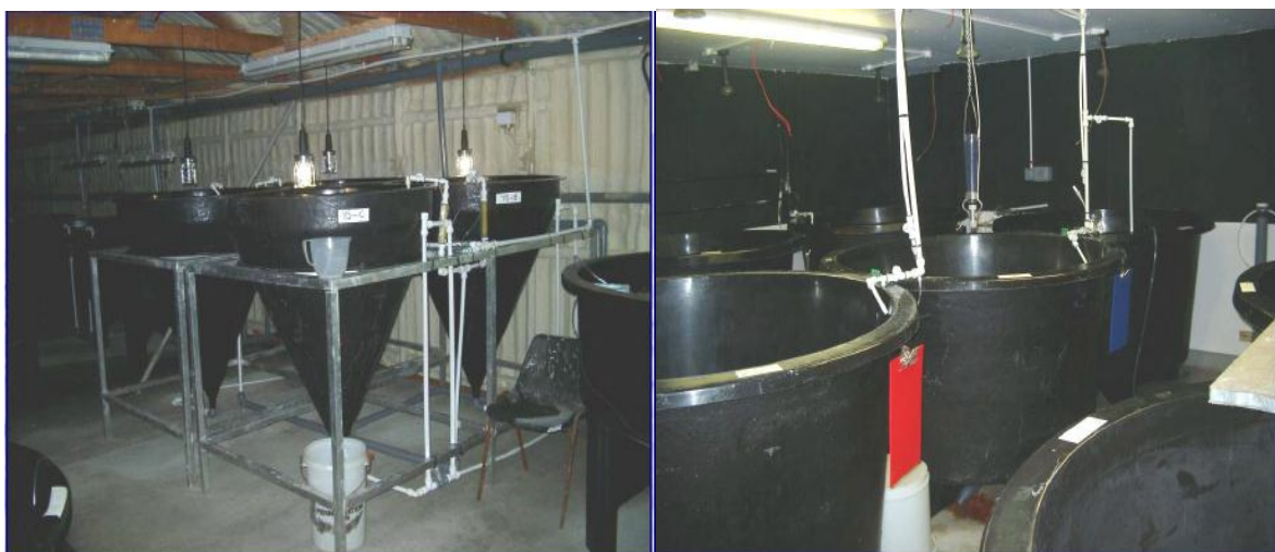
Figure 2.4.1.1: Conical -shaped up-welling incubation vessels (450 l, left picture) and larval rearing tanks small (1000 l, right picture), equipped with flow-, temperature control.
