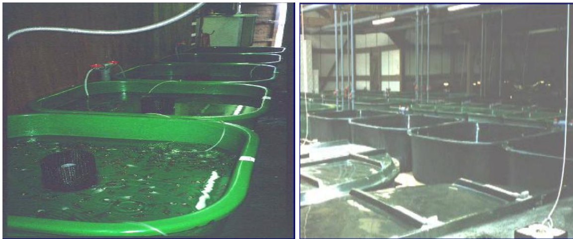
Figure 2.4.1.5: Halibut weaning and nursery tanks equipped with temperature control and aeration.
