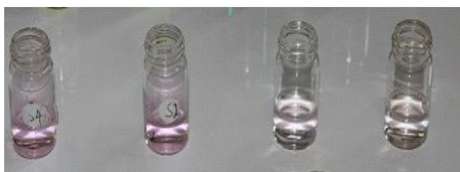
Figure 3.12 NO 2 -N determination: typical colours of prepared samples (highest concentration to the left).
