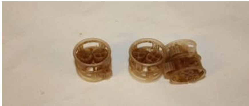
Figure 3.14 The mixture of the Kaldnes K1 and Pall Ring.
