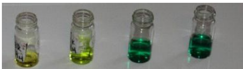
Figure 3.11 NH 4 -N determination: typical colours of prepared samples (highest concentration to the right).
