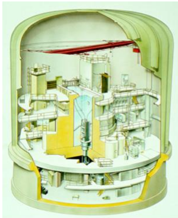
Figure 3. Cross section of the Petten High Flux Research Reactor in The Netherlands [18].
