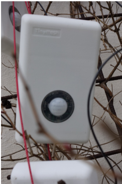
Figur 3.12 Tinymesh Room Climate Sensor kalibreres for CO 2 i noen rosebusker (Nilsen, 2013)
