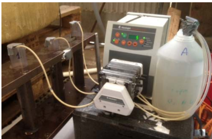
Figure 7: The three columns are loaded with feed solution by the use of a peristaltic pump.
