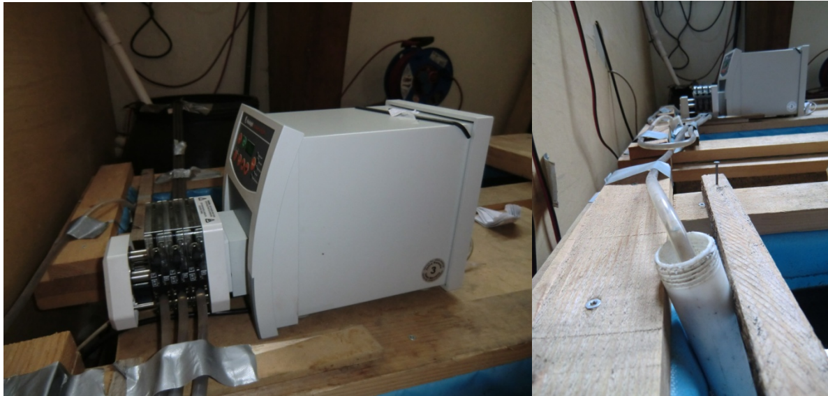
Figure 6: (Left): Peristaltic pump on top of the sedimentation channels. (Right): Greywater dosing system into the sedimentation channels. Hoses were led into tubes to stay stable.
