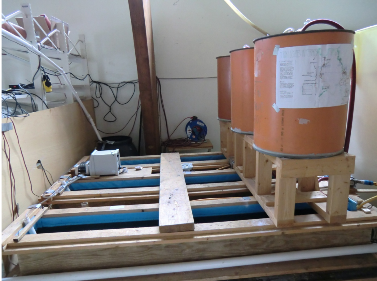
Figure 3: The experimental GWTP with the peristaltic pump in the middle of the sedimentation channels. Each channel is fed through equally long tubes.
