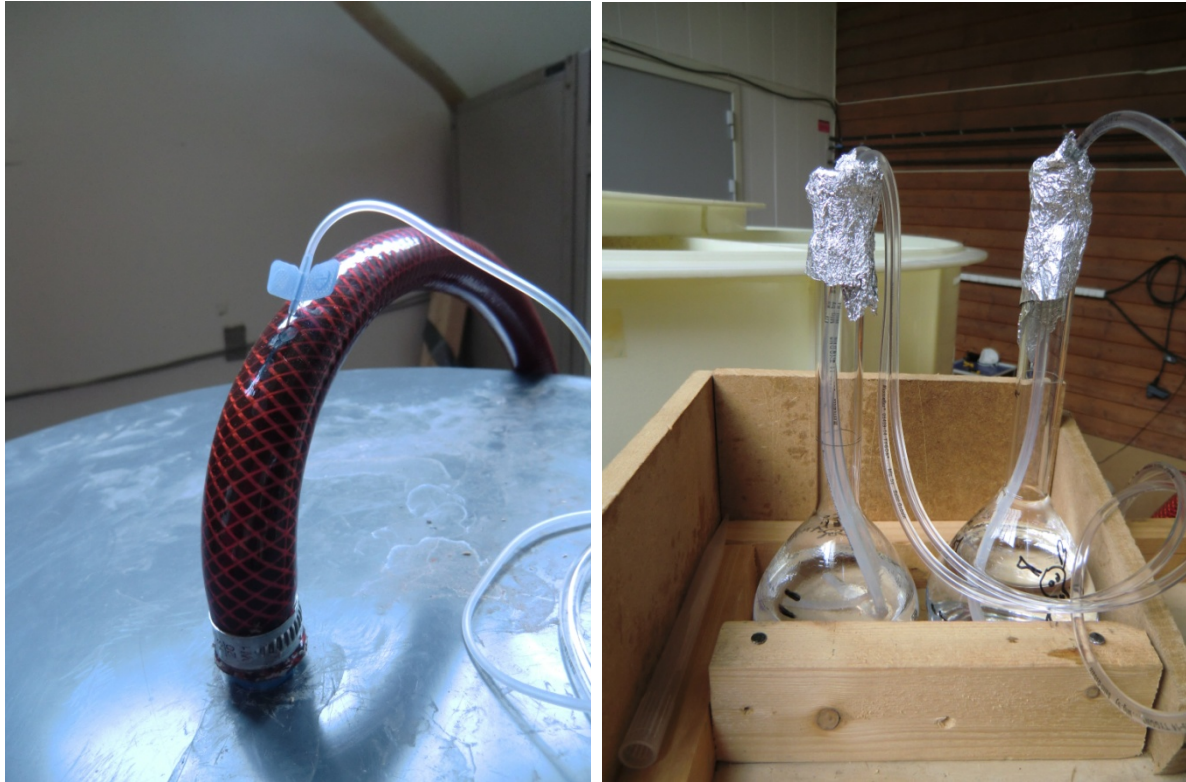
Fig. 5: (Left): The syringe needle at the end of the chemical solution hose pierces the filter hose just above the nozzle. (Right): The bottles containing the two chemical solutions, on top of the filters.
