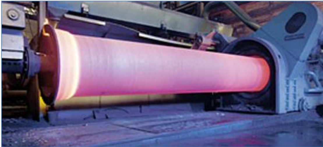
FIGURE 3.5 – A CAST IRON PIPE TAKES SHAPE (DUKTUS.COM 2012)
