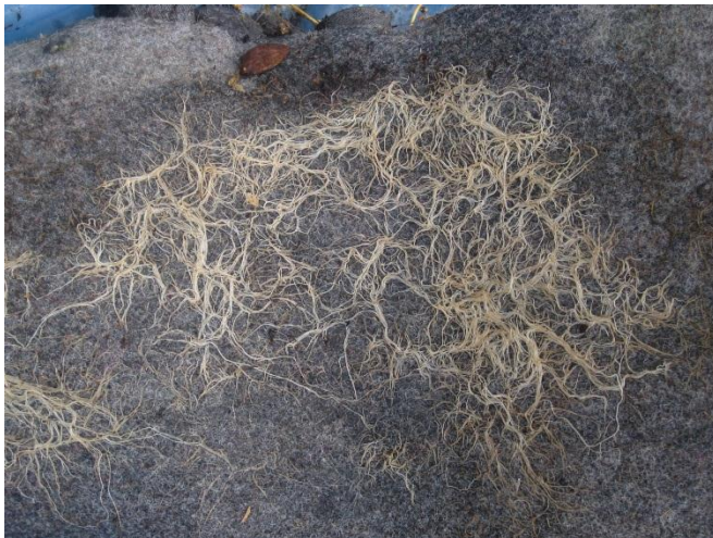
Figure 10 – Root establishment inside synthetic felt material (ZinCo SSM45)
