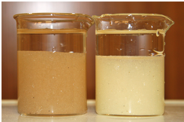
Figure 18: Colour change in resin (Photo: Marie Fauskrud)
