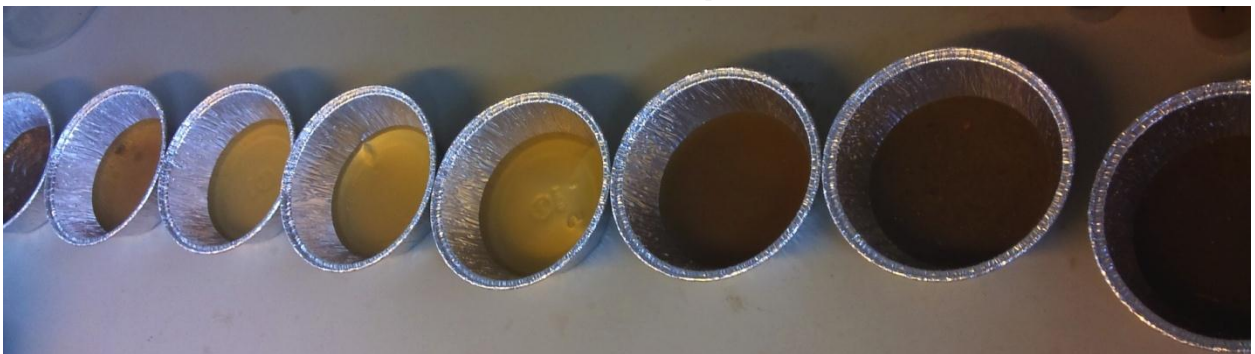
d. Clogging development after the drying period, this sustains for the filters toward the experiment end. Filtration slow down to 3-7 days and scum coverd at the top.
