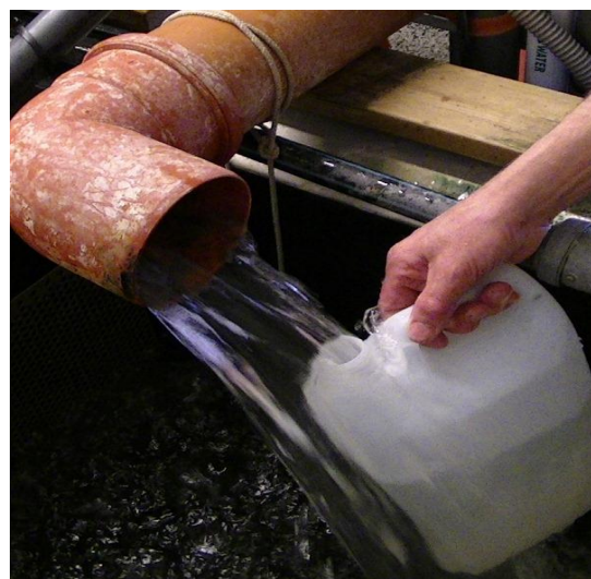
Figure 10: Spot where water sample after drum filter is taken (drum filter outlet pipe) (left). Water sample is taken by putting the canister under the water source that comes from outlet pipe from drum filter (right).
