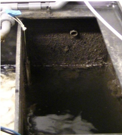
Figure 13: Chamber with water after MBBR (left). Outlet pipe from the drum filter inner side. Solids fasten to the pipe wall (right).
