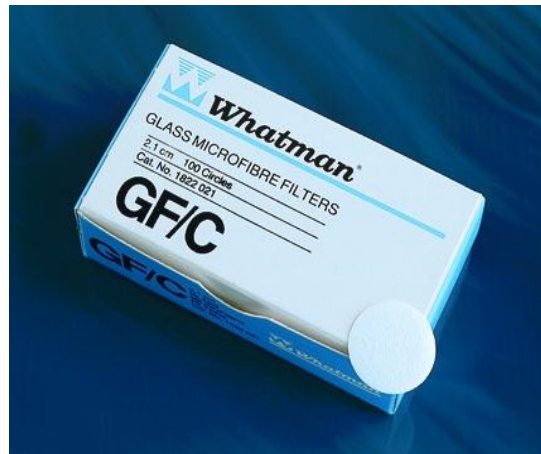
Figure 6: Digital drying scale for particle analysis (company Ohaus ®, model MB45) for calculating the weight of residue retained on the filter. Scale has the accuracy of 0,001 g (1,0mg), 0, 01% moisture and capacity 45g. Also, provide information about % of solids, time, temperature, weight, and drying curve (left) and Glass micro fiber filter 0,45 \mu\text{m} for fine particles (GF/C, company Whatman®) with good flow rates, high loading capacity and retention of very fine particles (right.)
