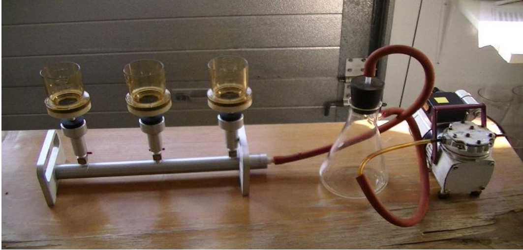
Figure 5: Filtering setup: glasses with the filter plate, Erlenmeyer bottle with side-arm socket and electric pump for supporting the vacuum.
