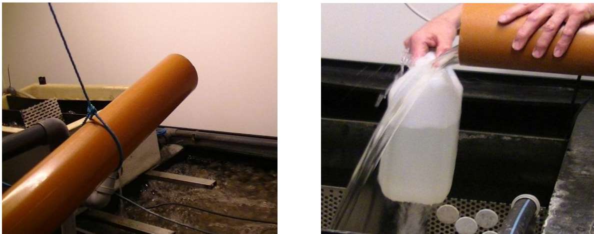
Figure 7: Fish tank outlet pipe, spot where the water sample before drum filter is taken (left). The tube is tilted down and held for 1 minute to “old” water flow out. After that time, 5 l canister was put under the tube and filled with the water (right).
