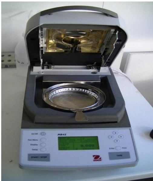
Figure 6: Digital drying scale for particle analysis (company Ohaus ®, model MB45) for calculating the weight of residue retained on the filter. Scale has the accuracy of 0,001 g (1,0mg), 0, 01% moisture and capacity 45g. Also, provide information about % of solids, time, temperature, weight, and drying curve (left) and Glass micro fiber filter 0,45 \mu\text{m} for fine particles (GF/C, company Whatman®) with good flow rates, high loading capacity and retention of very fine particles (right.)
