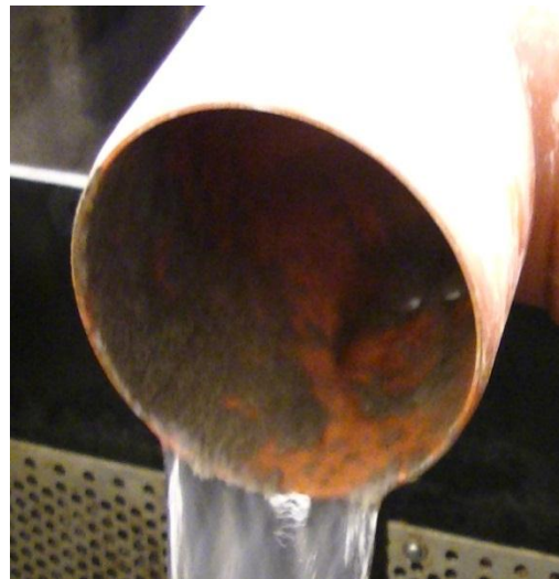
Figure 13: Chamber with water after MBBR (left). Outlet pipe from the drum filter inner side. Solids fasten to the pipe wall (right).
