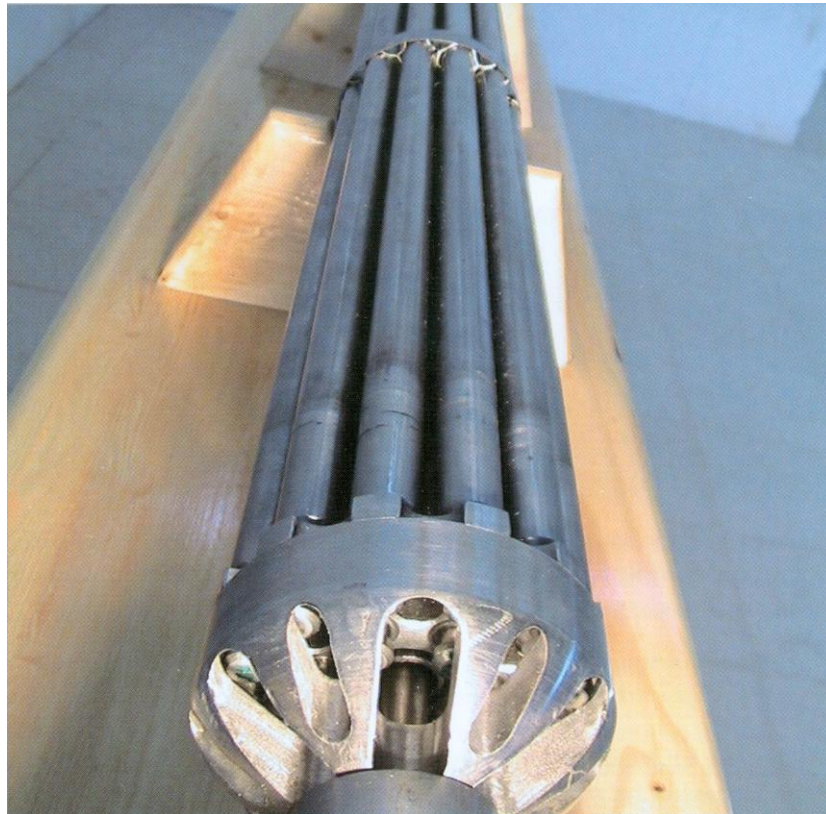
Figure 8-3. An RBMK-resembling fuel assembly displayed in a brochure from the AEOI about the nuclear industry in Iran [21].
