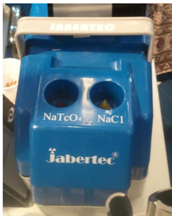
Figure 7-2. An Iranian-produced technetium generator displayed by the AEOI during the 55th Annual Regular Session of the IAEA General Conference in Vienna 2011. (Photo: Halvor Kippe.)
