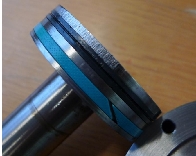
Figure 37, Shows damaged piston after dynamic test
