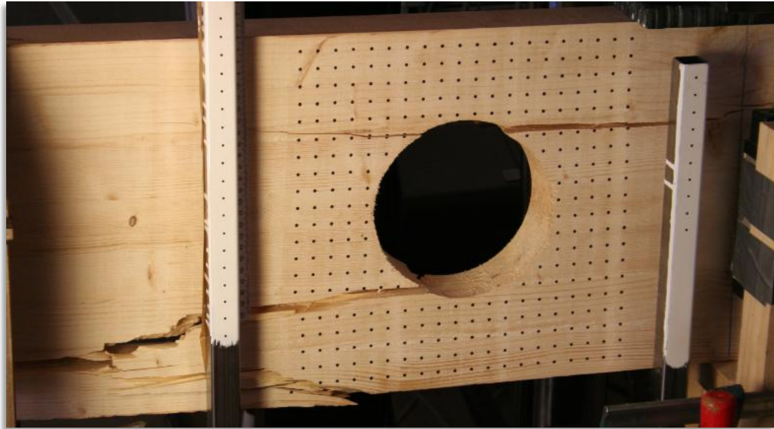
Figure 36: The measured grid at failure
