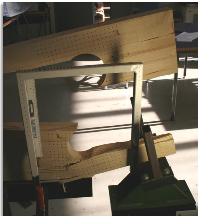
Figure 25: Beam 2A at failure
