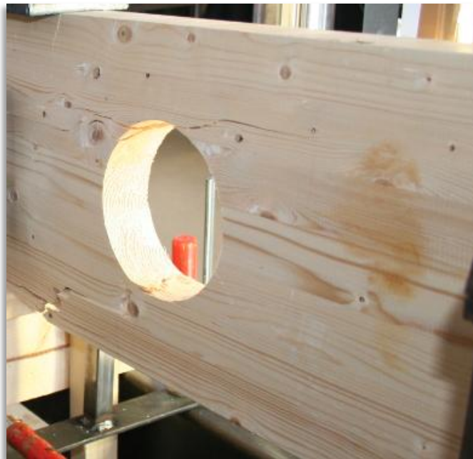
Figure 29: Knot in zone 2 and 3 on the back side of the beam
