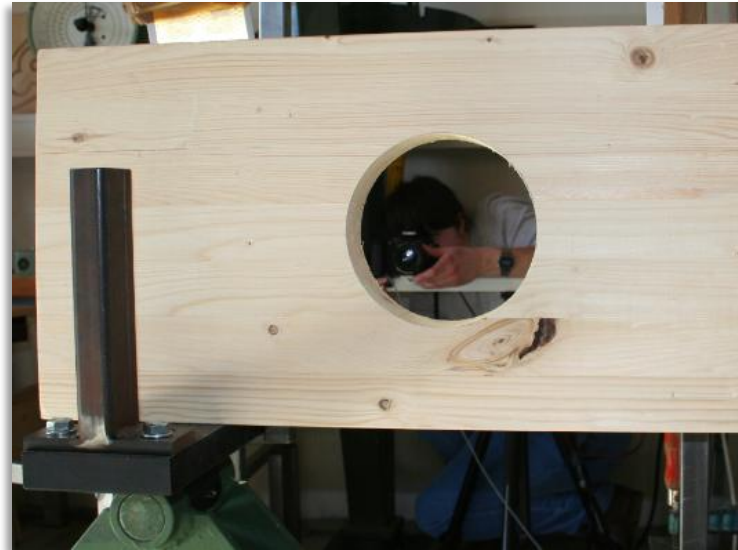
Figure 24: The back side of the beam. The knot is located in zone 3 in the grid
