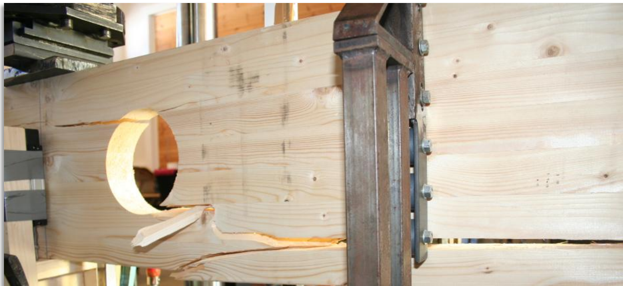
Figure 37: The back side of beam 5B. The knot to the right is located in zone 4
