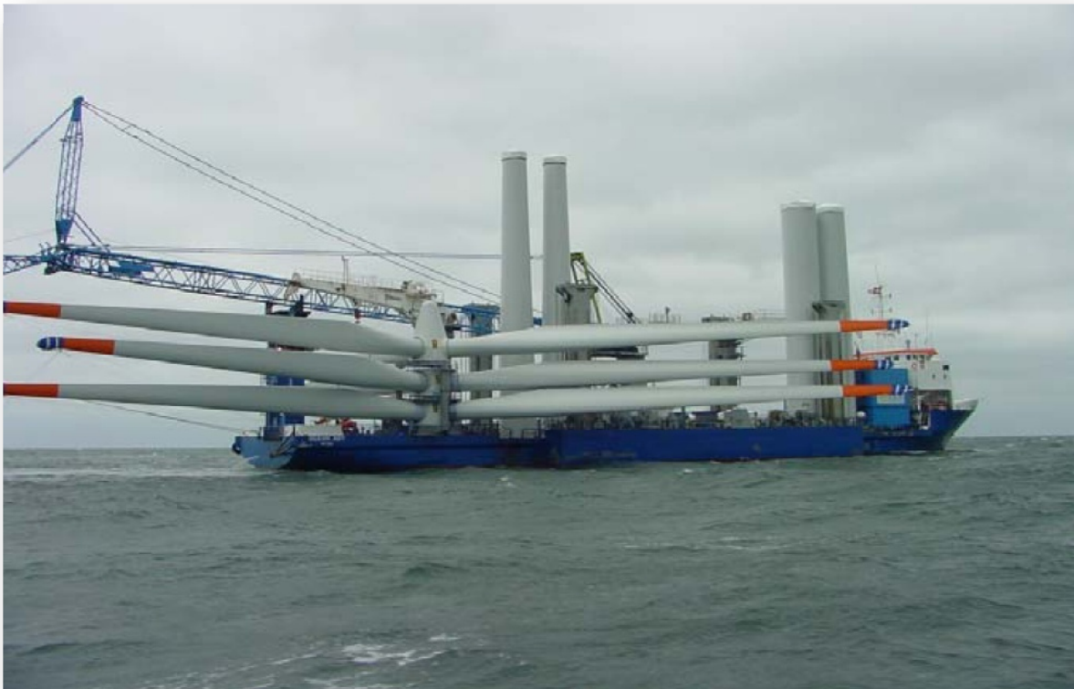
Figur 43: Rotorbladene er laget for horisontal utkraget transport (A2SEA AS 2007)
