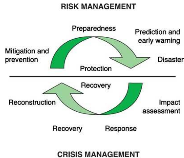
Fig 4.5: Disaster management cycle: This was first crafted by Wilhite, and has been extensively used to analyse the risk amelioration processes showing crisis management as a reactive process, while risk management is more proactive. Source: FAO, 2004
