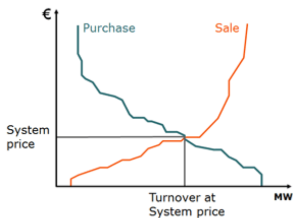
Figure 7: The system price is found where the aggregated demand and supply curve intersects. (Nord Pool Spot [9])
