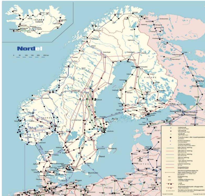
FIGURE 2.2 NORDEL TRANSMISSION GRID OF NORTHERN EUROPE, SOURCE: SWEDENERGY
