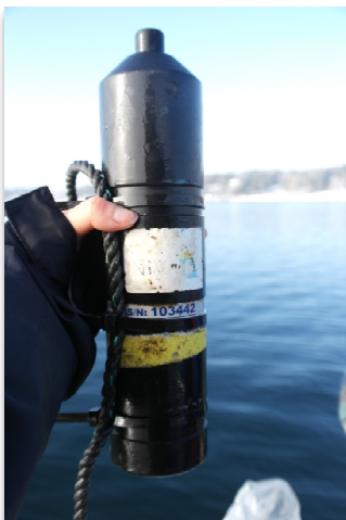
Figure 4. A) VEMCO VR2W stationary hydrophone, B) VR2W probability of detecting a signal (dashed lines: 95% confidence limits) estimated by range test (Dzadey In prep)
