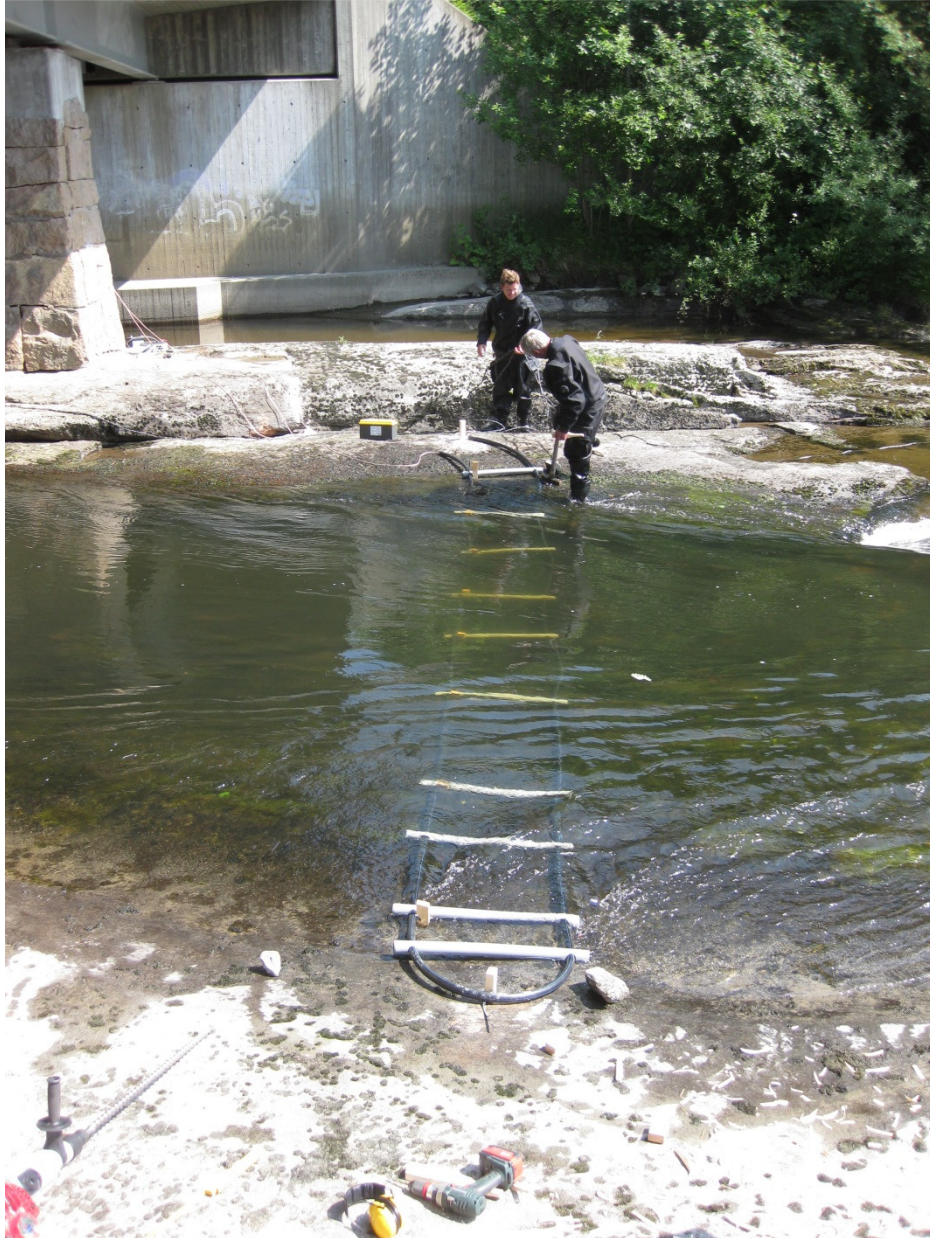
Figure 16. Installation of PIT antenna in Låkedalen.
