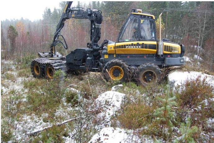
Figur 12. Ponsse Dual kombimaskin
