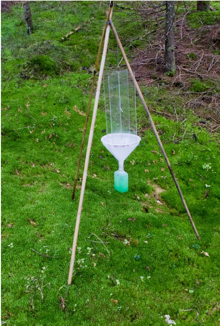
Figure 2. Tripod of slanted bamboo poles holding the interception trap. Plexiglas in a cross above the funnel with the storage container at the bottom. Flying beetles collide with the plexiglas and fall down into the funnel leading into the container with conservation fluid (photo: Jogeir Engeset Mikalsen).
