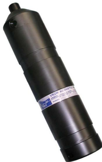
Fig. 4. VR2W Acoustic receiver (length: 308mm, diameter: 78mm) which were used to monitor lobster activity.
