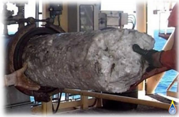
Figure 6: A gas hydrate plug (Hydrafact & University 2011).
