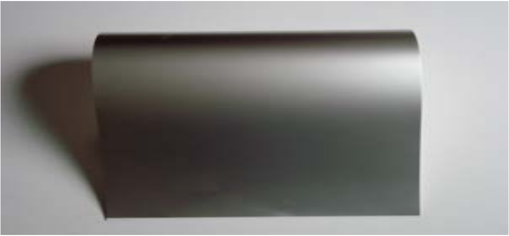
Figure 3.1 Paperboard blank laminated with aluminium and polyethylene
