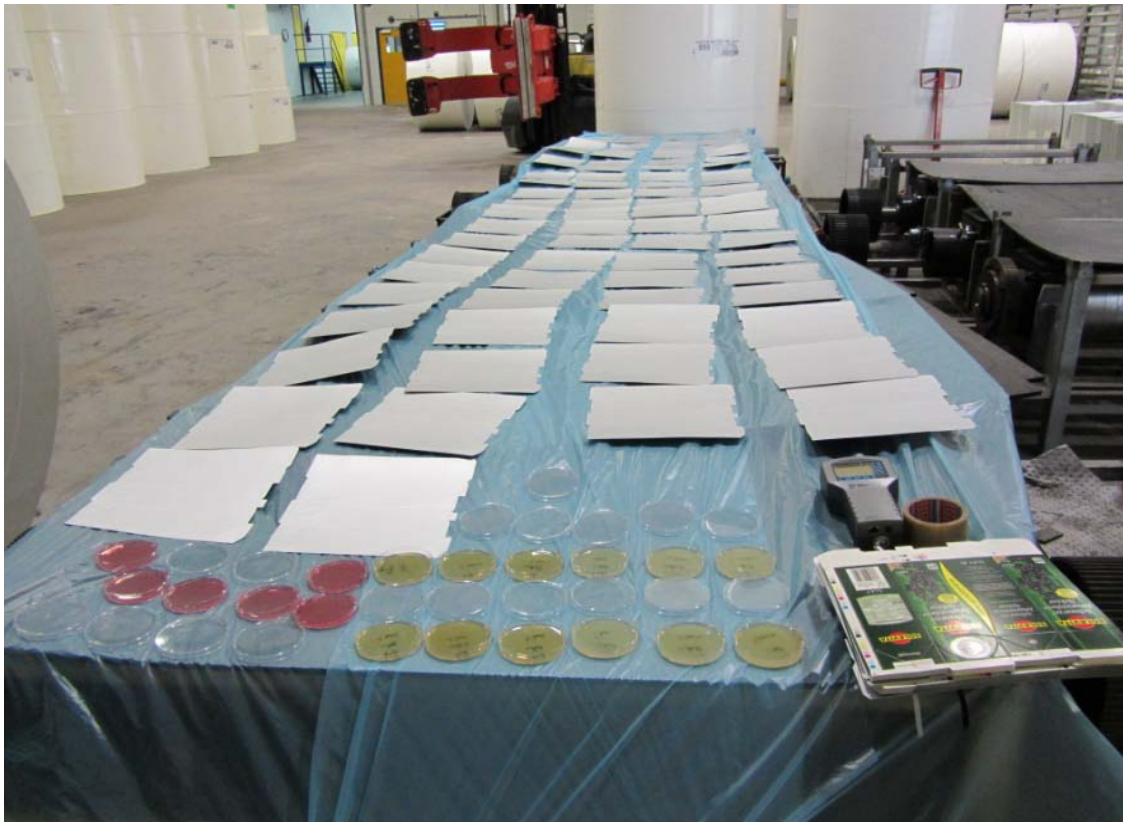
Picture 3.1 Exposure of flat blanks to ambient air in the storage halls at Terneuzen
