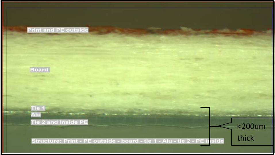
Figure 3.2a Cross section of the materials that make up the gable top carton
