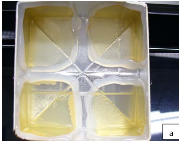
Figure 3.1 Cut carton bottoms with agar on corners. Note the glue frame around the corners restricting agar to the corners. a: Intact bottom (new method). b: Flat bottom (previous method). Growth on agar indicates survival of spores after d the decontamination process.
