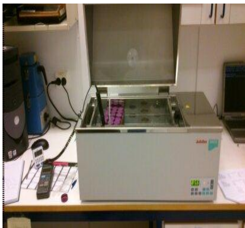
Fig. 8: Water bath with the samples. Here one can see the thermometer in a test tube. Used a stop watch to measure the time.
