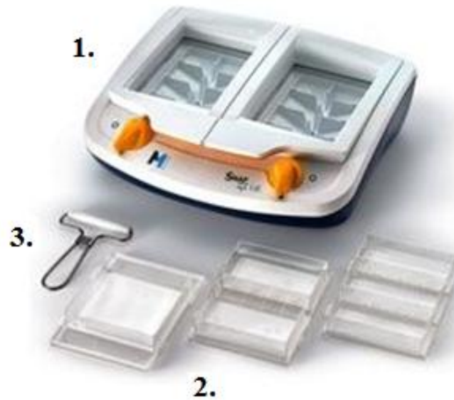
Figure 3.5: Illustration of the SNAP i.d. Protein Detection System. The figure illustrates all components in the SNAP i.d. Protein Detection System. The system (1) contains two blot holder chambers, each controllable with yellow vacuum switches. Different blot holders (2) can be used according to blot size and antibody hybridisation composition. The blot roller (3) is used to remove air bobbles between the blot holder surface and the blotted membrane. A description of how the device is used is given in the text. The figure is taken from the SNAP i.d. Protein Detection System protocol (Millipore).
