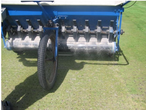
Figure 7: Applying mycorrhiza inoculum as surface dressing with a solid fertilizer machine (A), and raking the granules into holes from coring performed the previous day (B). Photo: Tatsiana Espevig.
