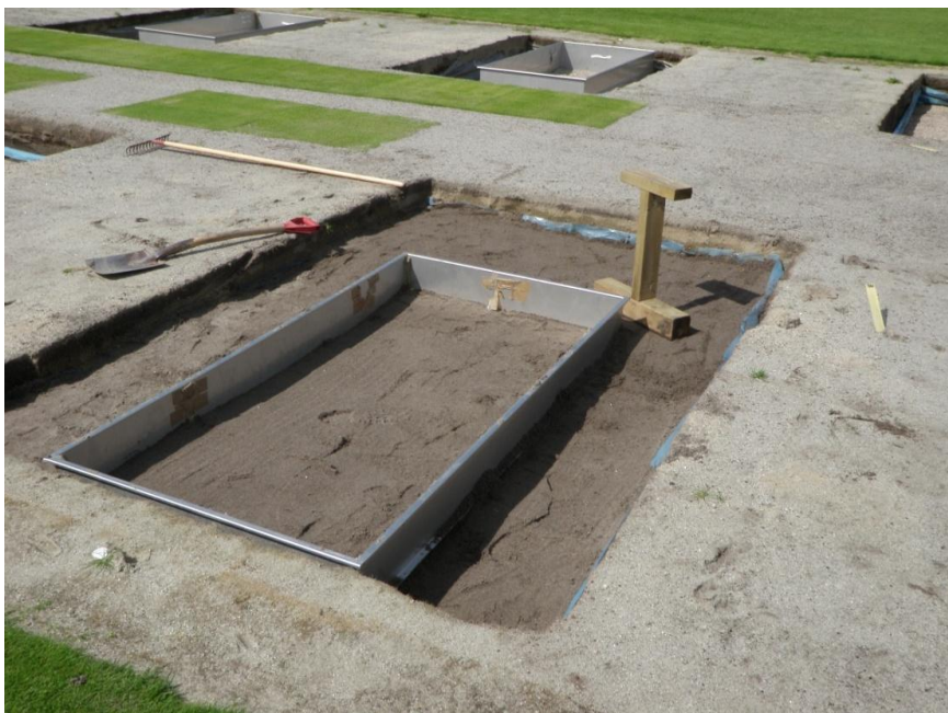
Figure 9: One of the plots before establishing the red fescue green in 2011. Old turf and growth root zone have been removed. The 0.4 m deep lysimeters are seen sticking up from beneath the ground in each plot. The tanks are 0.45 m deep with a drain line located in the middle. Photo: Trygve S. Aamlid.
