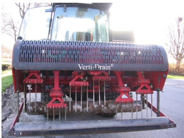
Figure 8: Tractor mounted VertiDrain machine used for deep ventilation.
