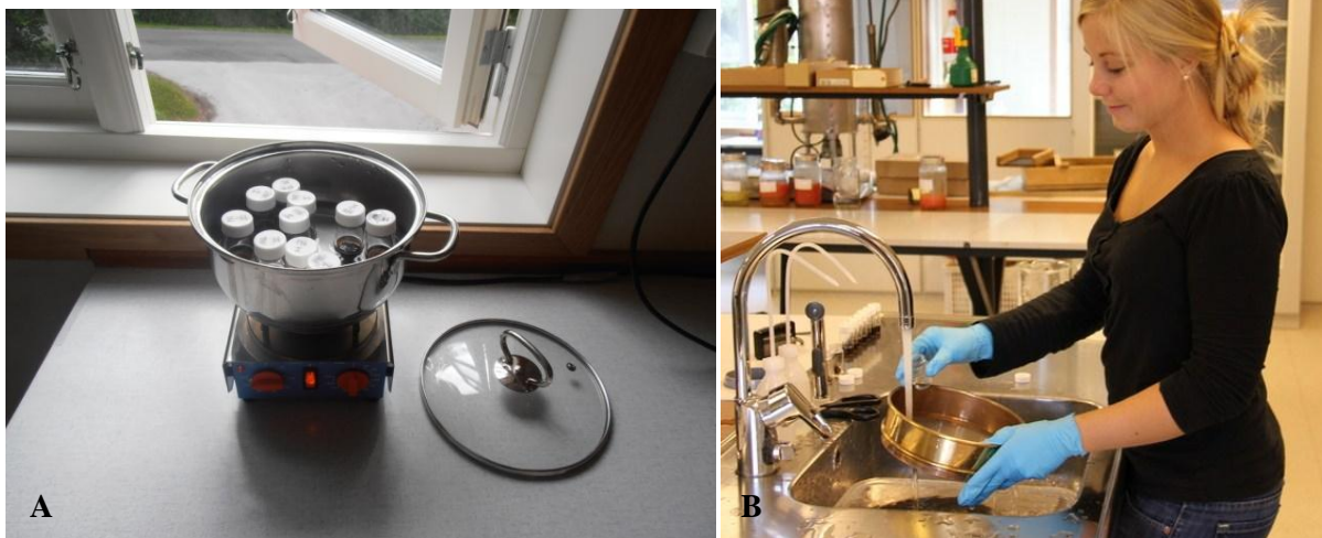
Figure 13: A: Boiling the roots with KOH in a water bath, to make their cells transparent and ready for staining. Flasks were cooled a couple of minutes before rinsing the roots. B: Rinsing roots free of KOH with the fine sieve. Photo: Tina E. Andersen (A) and Anne A. Steensohn (B).
