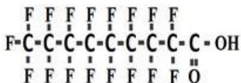
Figure 3: Chemical structure of PFNA ( C_9HF_{17}O_2 ).
