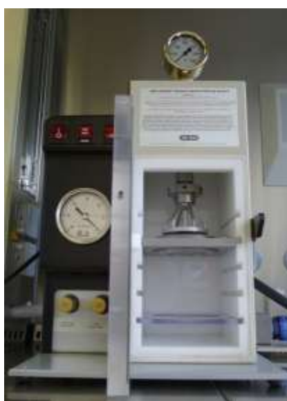
Figure 1.8: Biolistic PDS-1000/He Particle Delivery System. Helium enters from the top and vacuum is controlled to the left. DNA and explant is prepared and installed inside the bombardment chamber where Helium pressure in vacuum environment shoots the DNA-coated particles towards the explants.
