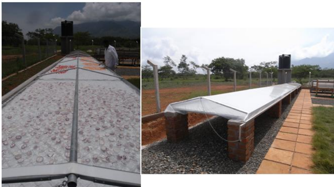
Figure 2: The tunnel dryer used by SUA, to the left filled with onions, tomatoes and carrots, and to the right without products.
