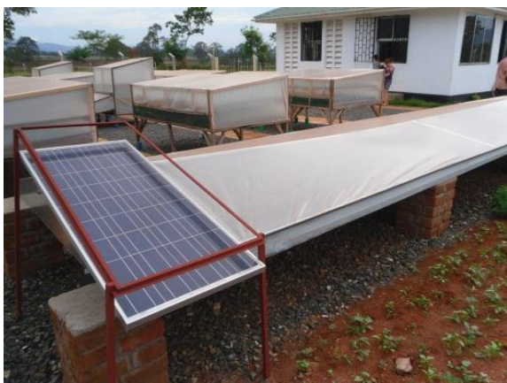
Figure 3. 3 The tunnel dryer with the solar module and the heating area.
