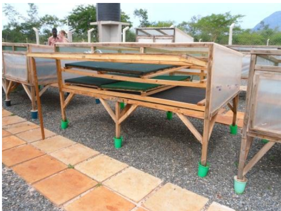
Figure 3. 1 Picture of a cabinet dryer. There is fly screen over the door for outlet of the air.
