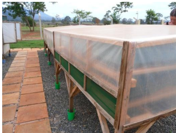
Figure 3. 2 Picture of a cabinet dryer from the back. The fly screen is for inlet of the air.
