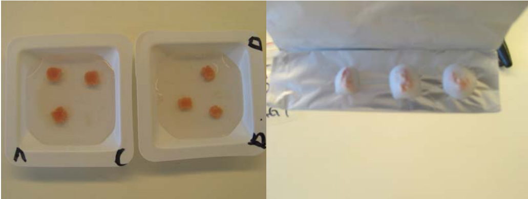
Figure 24: left: samples for FTIR and histology covered with O.C.T. compound. Right: Samples has been frozen in liquid nitrogen.
