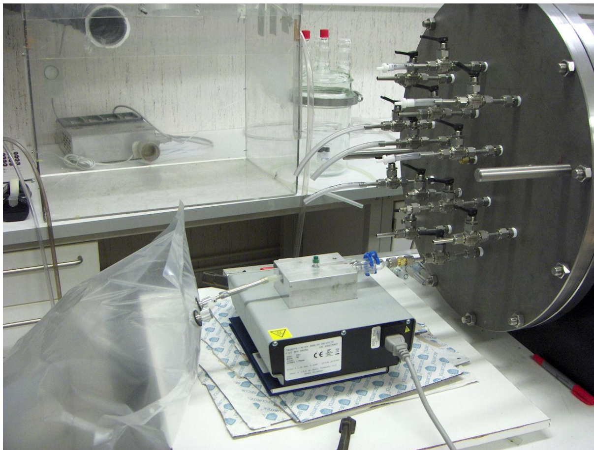
2.-1: An illustration of the set up for injection showing the injection unit (installed in the heating block) connected to the test chamber and a gas bag with N 2
