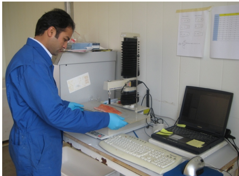
Fig. 3.2. Texture analyzer TA-XT2 (Stable Micro Systems Ltd, Surrey, UK) used for the texture measurements.
