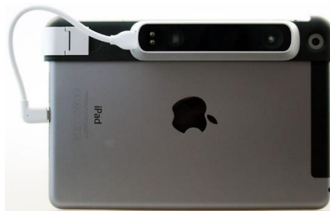
Figur 6-1. Rodin 4Ds 3D-skanner Structure sensor (Rodin4D 2016e).
